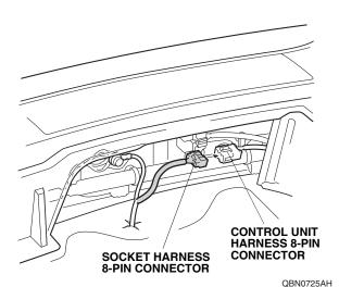
35. Secure the control unit harness 8-pin connector to the vehicle harness with one wire tie.
