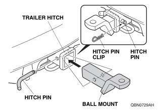
After the first 600 miles (1,000 km) of towing, have your Acura Dealer re-check the tightness of the trailer hitch bolts.
