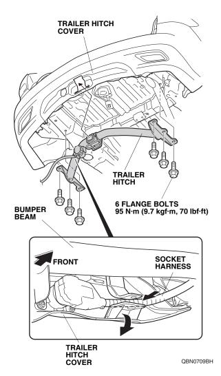
12. Torque the six flange bolts to 95 N·m (9.7 kgf·m, 70 lbf·ft).
