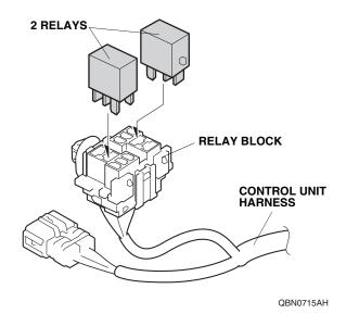
22. Route the control unit harness along the vehicle harness, and attach the control unit harness relay block to the vehicle panel.
