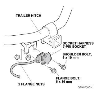
11. With the help of an assistant, position the trailer hitch on the vehicle and loosely install the six flange bolts.
